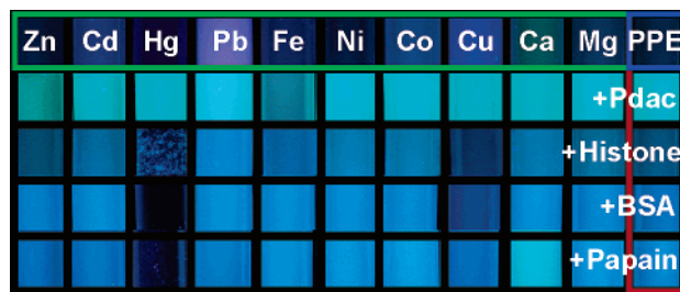
Figure 1. Addition of metal ions to PPE 1 in the absence and the presence of cofactors. Blue box: PPE 1 (all samples, 5 \mu M, \lambda_{\text{max}} abs 428 nm). Green box: 1 in the presence of different metals (metal concentration: 0.4 mM). Red box: 1 ·cofactor (cofactor concentration: 5 \mu M). Boxed data are controls. The picture shows the fluorescence of different samples under a hand-held UV light ( \lambda_{\text{max}} 365 nm). Metal cations are in the +2 oxidation state, with the exception of Fe, which is Fe 3+ .
